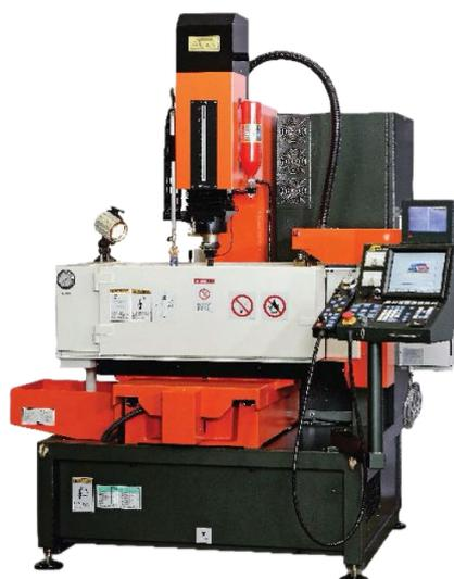
ELETTROEROSIONI A TUFFO ANCHE CNC
